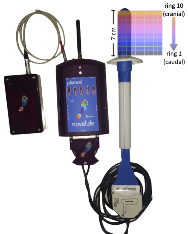
Fig. 1. Instrumented sensor probe: Pliance® System (Novel, Munich, Germany) including (from left to right) battery, multi-channel analyzer and intravaginal probe: Ertacetal® cylinder covered with capacitive transducers placed in a matrix configuration (10 × 10).
